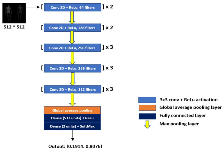
Fig. 2 The architecture used in the study. Pre-processed BS scans resized to 512 * 512 dimensions were provided as input to the network. The network outputs a probability score for presence and absence of metastasis on BS images. X= block repetitions, Conv = Convolution kernel, ReLU = rectified linear unit, 3 x 3 = the size of the 2D CNN kernels
